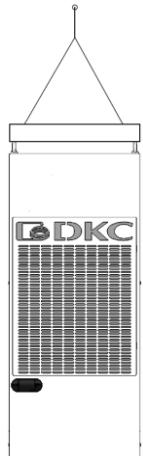
The coolers may be mounted inside or outside the enclosure. The cooler must always be installed in upright position (with the compressor in the bottom) with the maximum standoff from the upright position equal to 2°.
